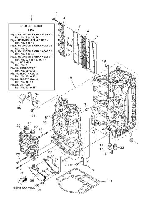
FIG. 3 CYLINDER & CRANKCASE 1
