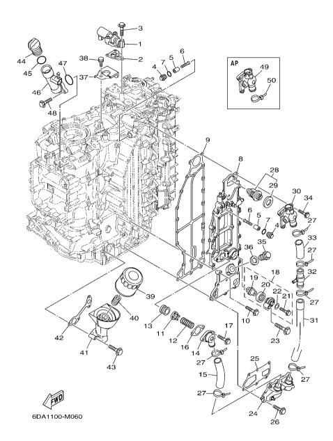
FIG. 6 CYLINDER & CRANKCASE 3
