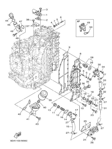
FIG. 6 CYLINDER & CRANKCASE 3
