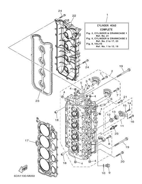
FIG. 5 CYLINDER & CRANKCASE 2
