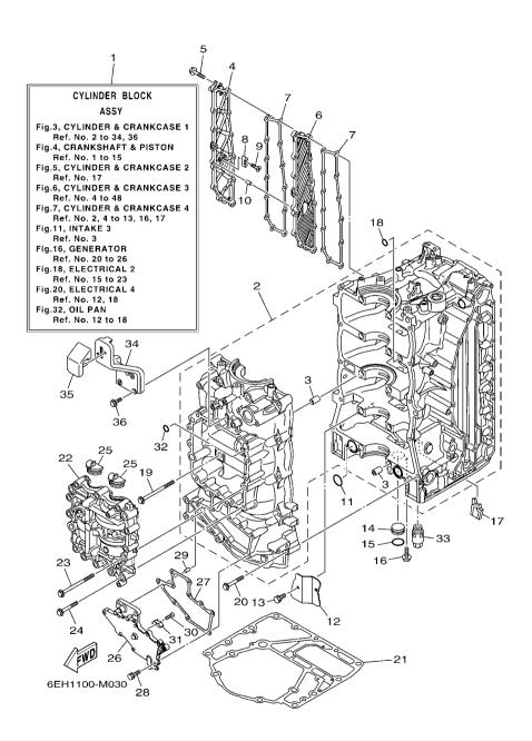
FIG. 3 CYLINDER & CRANKCASE 1
