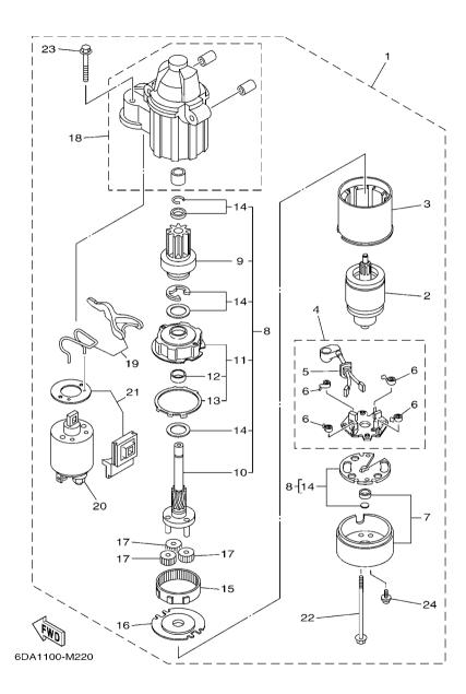
FIG. 22 STARTING MOTOR
