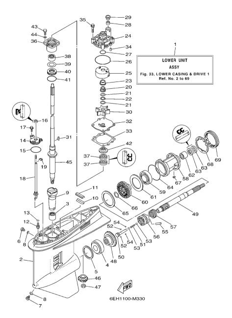
FIG. 33 LOWER CASING & DRIVE 1
