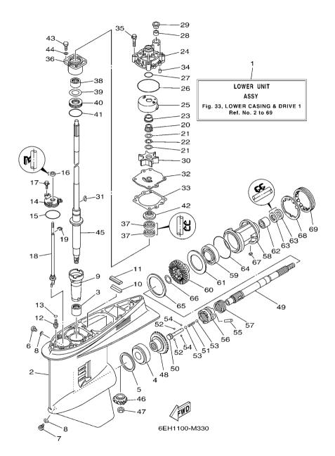
FIG. 33 LOWER CASING & DRIVE 1
